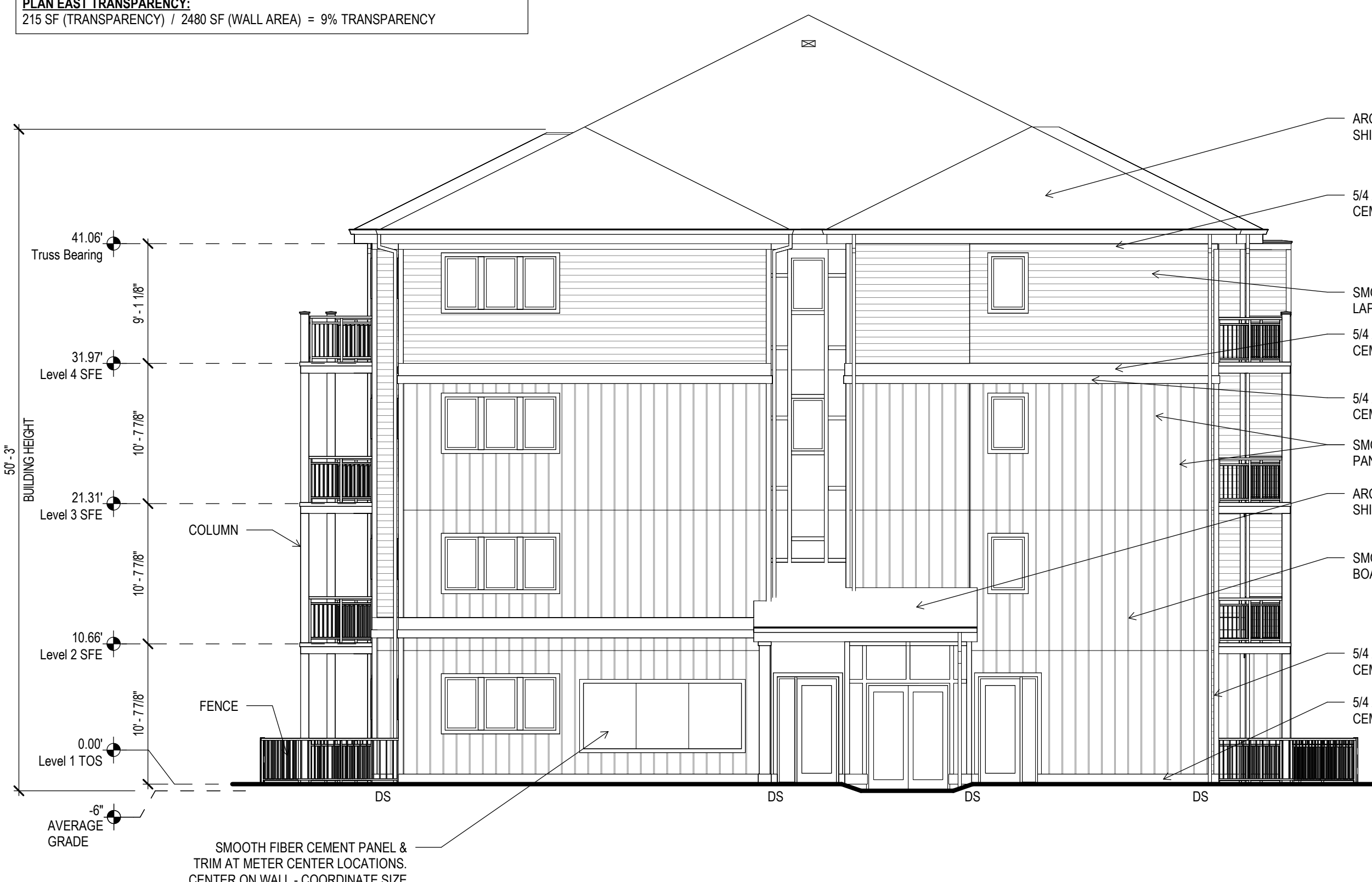
3 BUILDING 2, 4, 6 - SIDE ELEVATION LD-4 1/8" = 1'-0"
