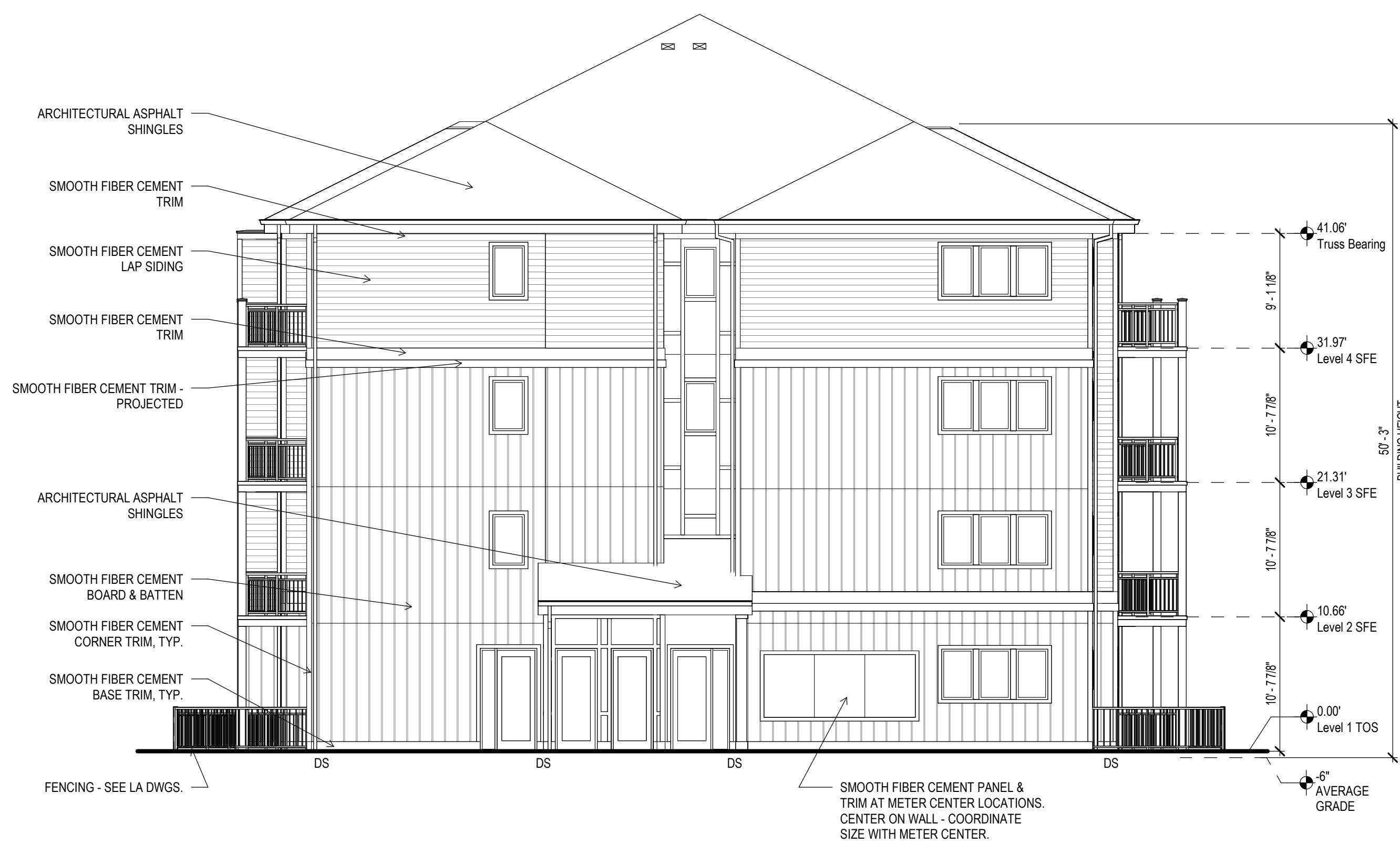
4 BUILDING 2, 4, 6 - SIDE ELEVATION LD-4 1/8" = 1'-0"
