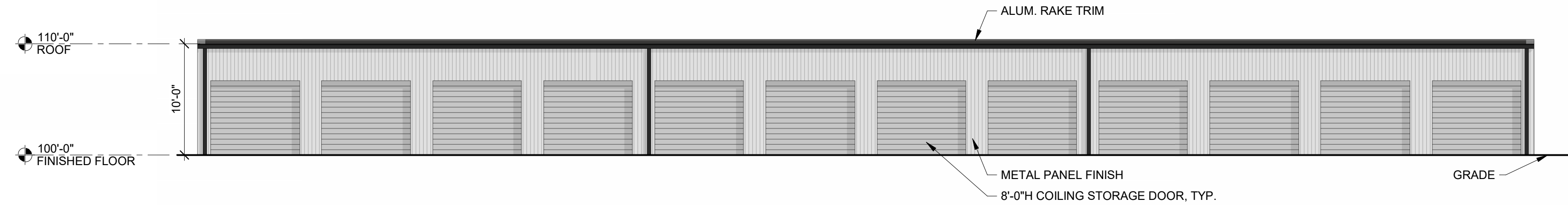
1 BUILDING 4 ELEVATION - FRONT A2.03 1/8" = 1'-0"
